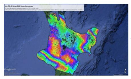
LEFT: This month's image has been provided by Ian Hamling. It shows a recent interferogram over the North Island made by ALOS-2. This interferogram uses the ScanSAR mode on ALOS-2 which enables the formation of interferograms approximately 400 km x 400 km
