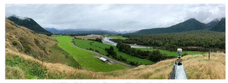
Static GNSS was utilised at the beginning of the project to establish a robust control network over the site.
