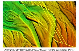
banks when determining water boundaries. Geo-referenced aerial imagery and a 3d terrain model was utilised to capture river boundaries. The use of the fixed wing UAV provided significant time savings with the capture of approximately 10km of water boundaries.
