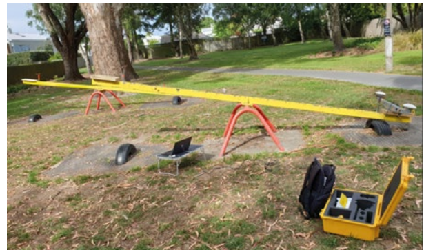
Left: Car-based testing of the BX992. Credit: G Chisholm Right: See-saw-based heave testing of the BX992. Credit: G Chisholm
