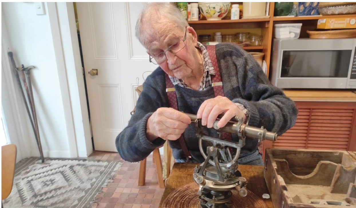
Photo caption: Bruce Alexander demonstrating a Wye theodolite in recent times. His other one, a Troughton and Simms that he bought ex-NZ Railways in 1955 was a life-long pride and joy as well as a tool of trade. Into his 90s he jumped at excuses to assemble it, and regale listeners how it could read to 10 seconds of an arc whereas some modern instruments could only manage 20 or 30.
