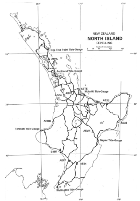
Figure 5. NZ North Island precise levelling networks, tide gauges and LVD junction points
